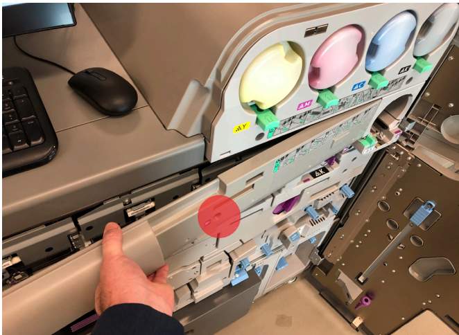
Replace top cover with (2) screws highlighted.
