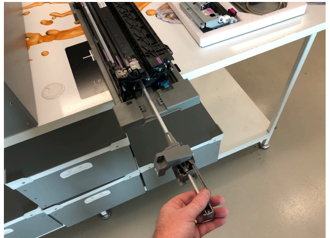
Completely remove securing rod from drum assembly.
