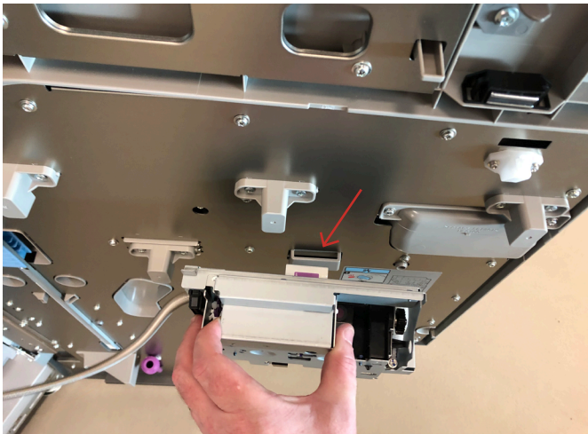
Place toner hopper on slot in RHS door.
