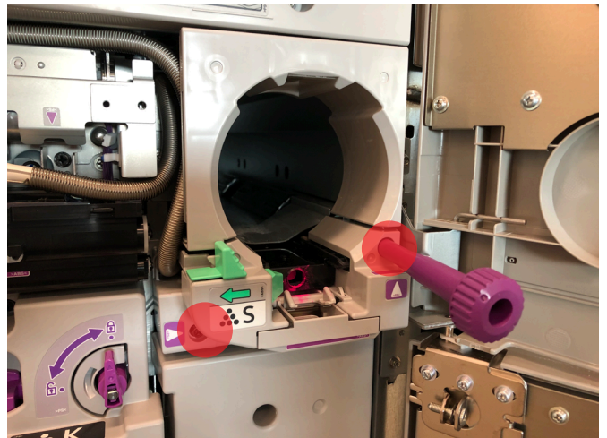
Remove bottle holder (2) screws as pictured.
