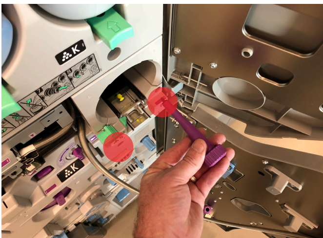
Attach bottle holder (2) screws as pictured above.
