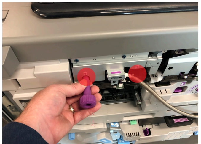
Attach new toner hopper (2) screws as pictured.
