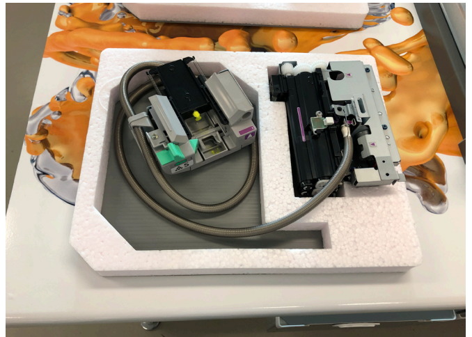
Grab new 5th colour toner hopper and bottle holder assembly.
