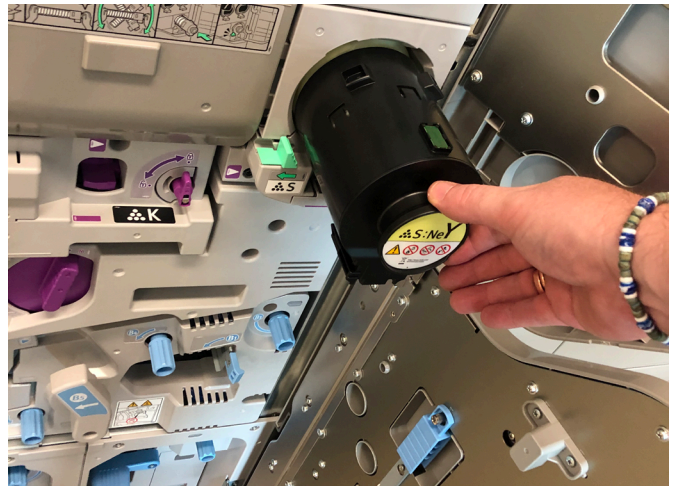
Load "new" 5th Colour Toner cartridge.
