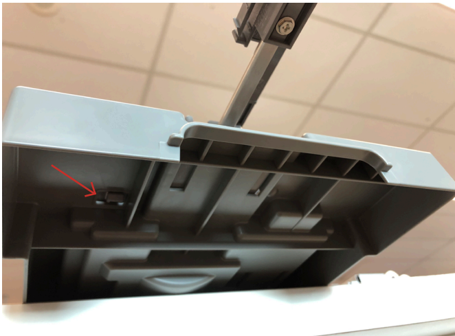
On underside of tray release catch.
