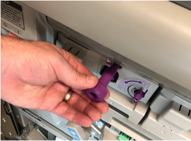
Secure drum assembly as pictured (1) screw.
