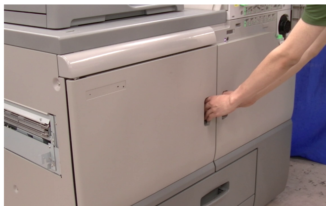
18. Open machine front covers .
