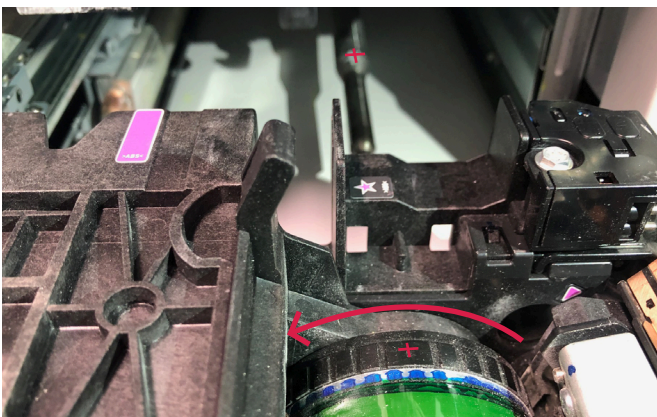
71. Turn drum counter-clockwise only to align positive symbols on both drum and spindle.
