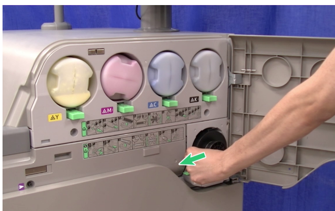
15. Remove "Dummy" toner bottle.
