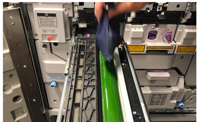
72. Lubricate drum with powder provided.
