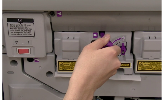
20. Using supplied purple "Hex Tool", remove bolt as pictured.
