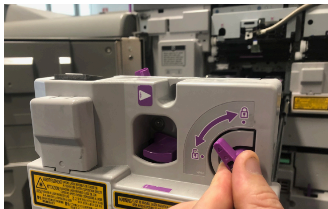
74. Lock Drum Cleaning Unit.
