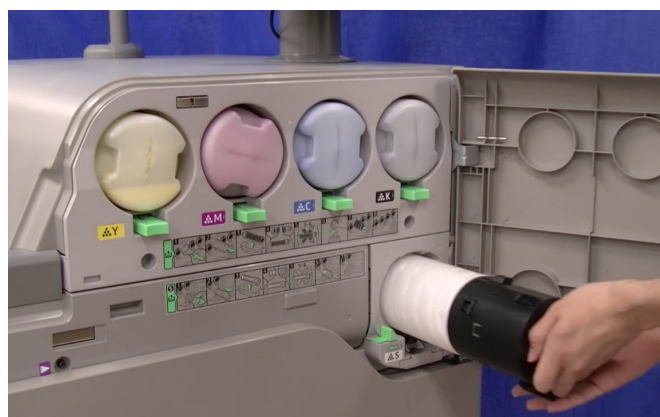
16. Insert "Catchment" Toner bottle supplied with Toner pump.
