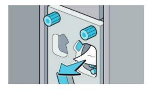
6. Turn the knob Kc4 to clockwise for 20 to 22 times.
