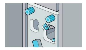
2. Turn the knob Kc1 to counterclockwise for 20 to 22 times.
